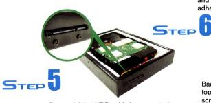
Be careful that HDD cable is connected completely before you close the top. Cable should not get any pressure by closing the top
